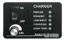
A remote control panel may be connected to the battery charger using a 9-pin D-connector that attaches to the side of the battery charger. The remote control panel and D connector are part of the remote control option. The remote control panel allows the unit to be operated remotely as well as duplicating all the diagnostic indicators and audible alarm
