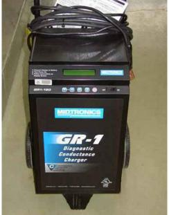
Minimum Battery Voltage (OCV) start: default 0.5 VDC Diagnostic time: 1-3 minutes
