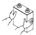
USE EDGE OF CELL WHEN POSITIONING BATTERY
